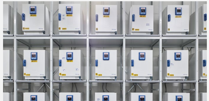
Ovens in the Trelleborg Sealing Solutions Material Laboratory are used to test materials for compatibility with CIP media.
